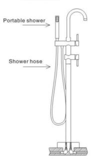
Diverter: switch water between spout & hand shower. Turn left for hand shower, while turn right for spout.
