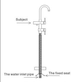
3、.Install the flexible hose now and ensure the flexible hoses are hand tightened into place (DO NOT USE SPANNER TO TIGHTEN AS IT CAN DAMAGE THE O-RING). The flexible hoses are to be fitted into the correct inlets for hot water and for cold water.
