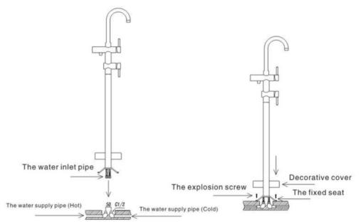
5. Connect another side of the flexible hose to the water supply pipe. Make sure they are to be fitted into the correct outlets for hot water and cold water.
